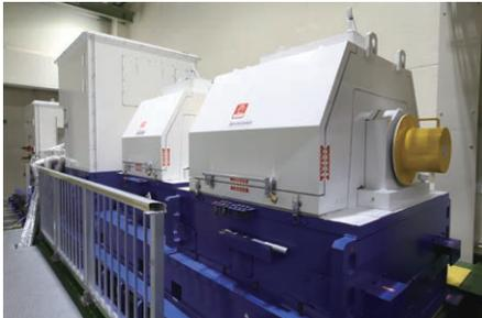
Transient Dynamometer Testing Equipment
